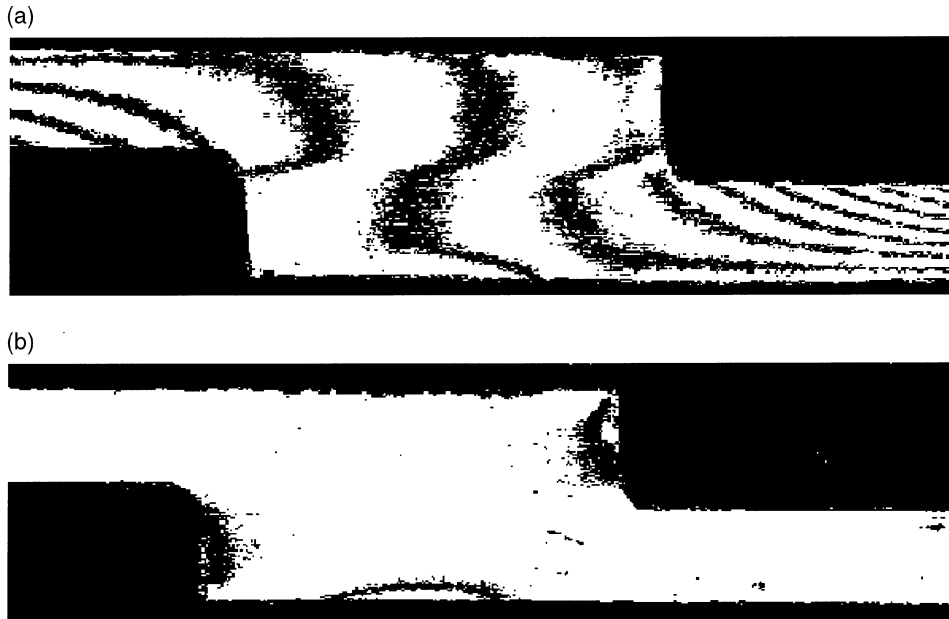
Fig. 8. Fringe patterns without alignment (left) and with alignment (right).
